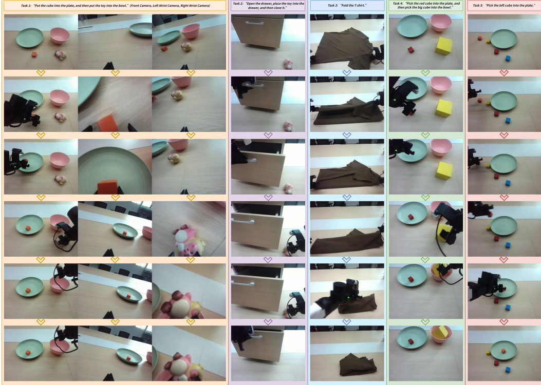
Figure 2: Real-world Manipulation Workflows and Visualizations for Tasks 1–5. Each task panel illustrates the initial setup and CogVLA’s execution process based on the natural language instruction. For Task 1, multi-view observations from the Front Camera , Left Wrist Camera , and Right Wrist Camera are provided to capture dual-arm coordination. For Tasks 2–5, representative frames from the Front Camera highlight key manipulation stages. These visualizations support interpretation of task complexity and grounding behavior.
